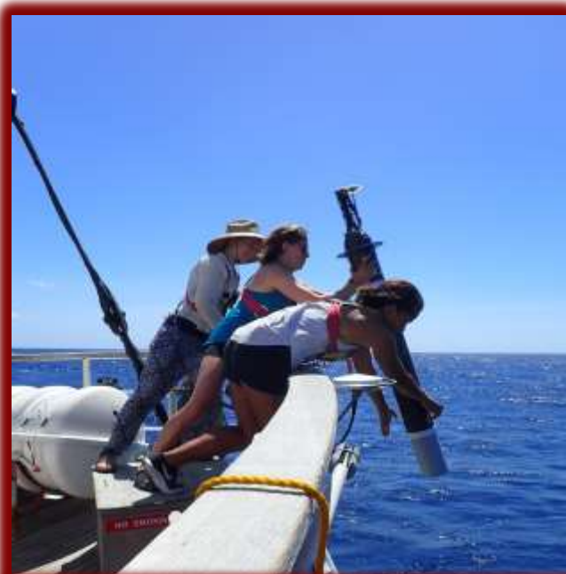
Casidhe Mahuka deploying an oceanographic instrument that measures temperature, conductivity and depth with shipmates onboard the Robert C. Seamans.
